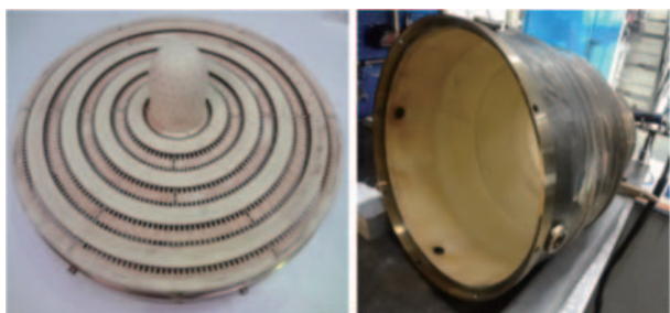
Fig. 19 Pictures of combustor parts after the test (0.55 MMX)
