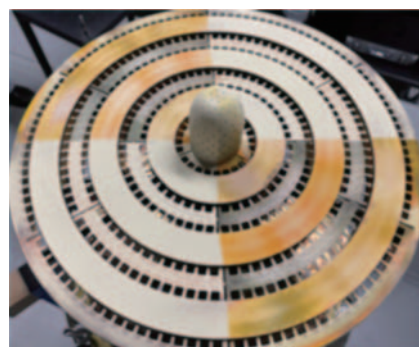
Fig. 29 0.8MMX burner module after engine demonstration tests
