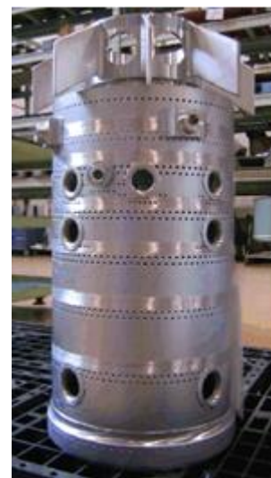
Fig. 4 Single can type combustor
