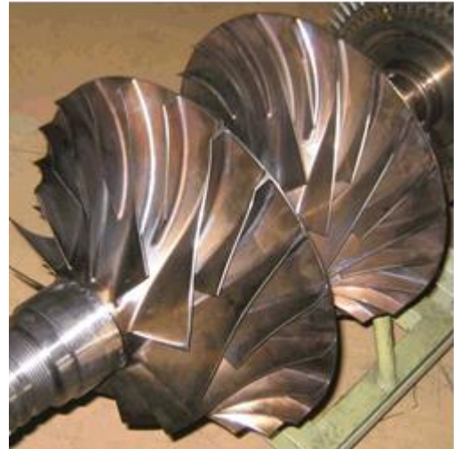
Fig. 3 Two stage centrifugal compressor
