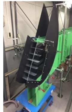
Fig. 1 Test section of linear wind tunnel
