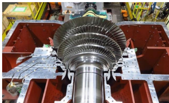
Fig. 1. A four-stage scaled model steam turbine
