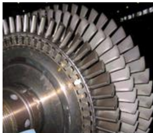
Fig. 7 Three stage axial turbine
