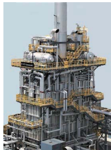
Fig. 6 Heat Recovery Steam Generator
