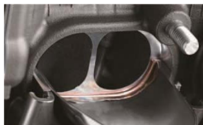
Fig. 19 Shape of exhaust gas outlet
