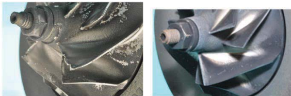
(a) No surface coating (b) With surface coating
