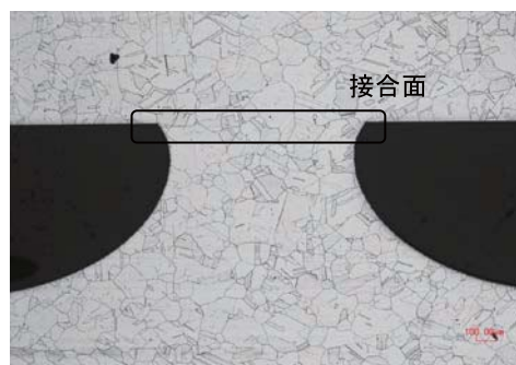
Fig. 12 Example of Cross section observation (SUS316L)
