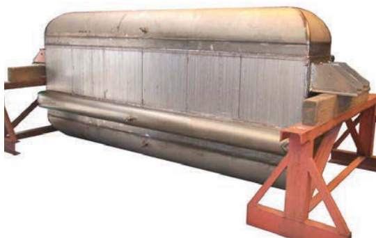
Fig. 13 Large scale Stainless steel heat exchanger with Multiple cores welded into single block
