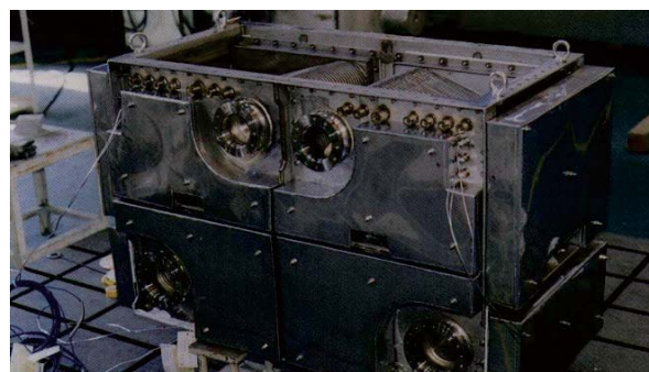
Fig. 7 Recuperator for Ceramic Gas Turbine
