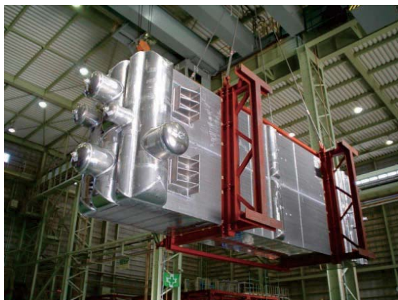
Fig. 5 Main heat exchanger for Air separation unit
