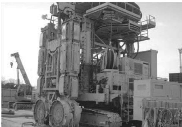
Fig. 8 Excavator of slurry wall
