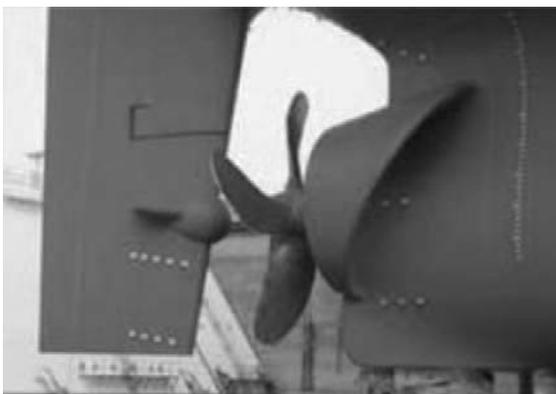
Fig. 3 SURF-BULB and SSD
