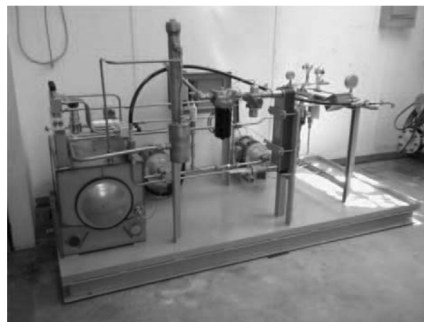
Fig. 9 Oil-gas mixture supply system for the seal test rig
