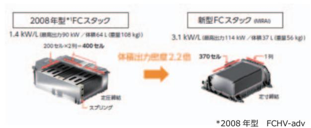
Fig.12 FC Stack comparison with 2008model
