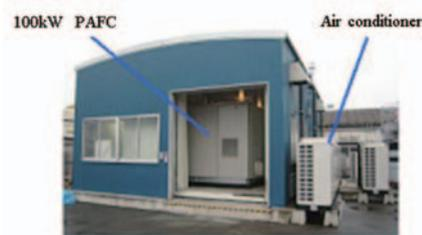
Fig. 5 The appearance of the environmental test room
