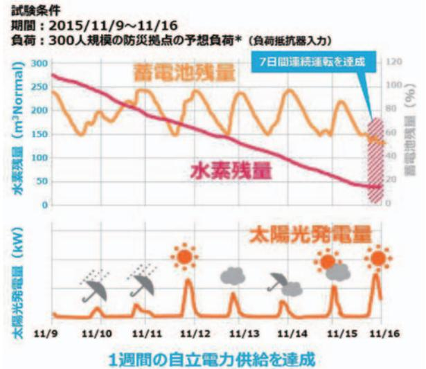
Fig. 5 Example of demonstration result of the one-week stand-alone operation
