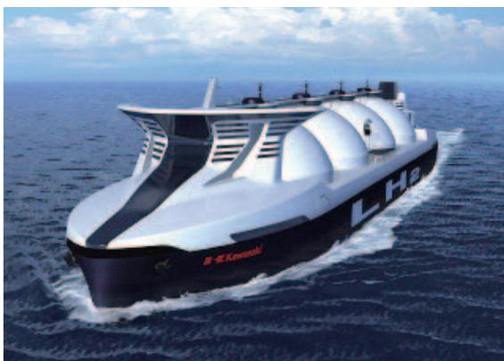
(c) Liquefied Hydrogen Carrier Ship (160,000 m<sup>3</sup>)Fig. 2 Feasibility study on CO<sub>2</sub> free hydrogen supply chain
