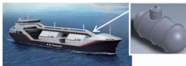
Fig. 4 Image of liquid hydrogen carrier and tank
