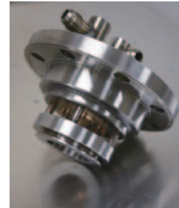
Fig.12 Supplemental burner for natural gas and hydrogen dual gas fuel
