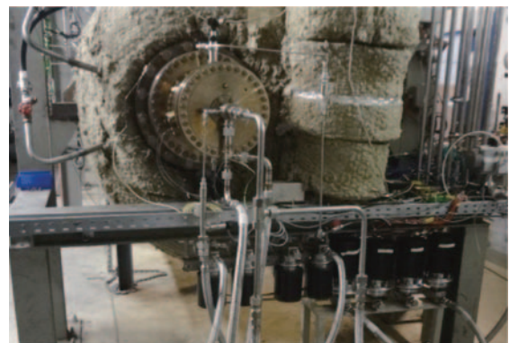
Fig.10 Hydrogen combustion test and investigations of NO x characteristics in high pressure conditions at RWTH Aachen University, Germany
