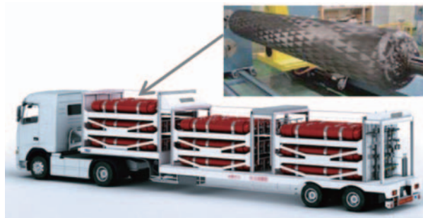
Fig. 5 Hydrogen gas carrier with 45MPa gas bottles
