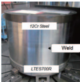
Fig.17 Rotor Dissimilar Welding (9),(10)
