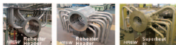
Fig.13 Reheater, Superheater Header Mock-ups (5)
