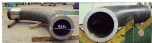
Fig.12 Boiler Pipe Bending Test (3)
