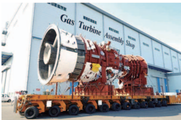
Fig. 2 1,600°C J-type gas turbine
