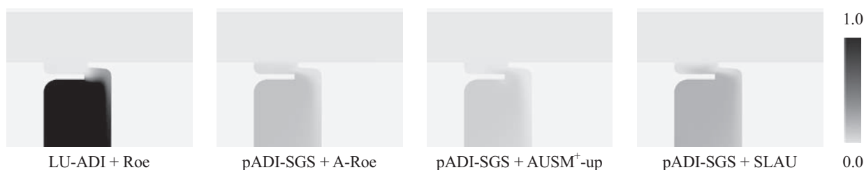
Fig. 3 Comparison of Seal Efficiency by Each Schemes
