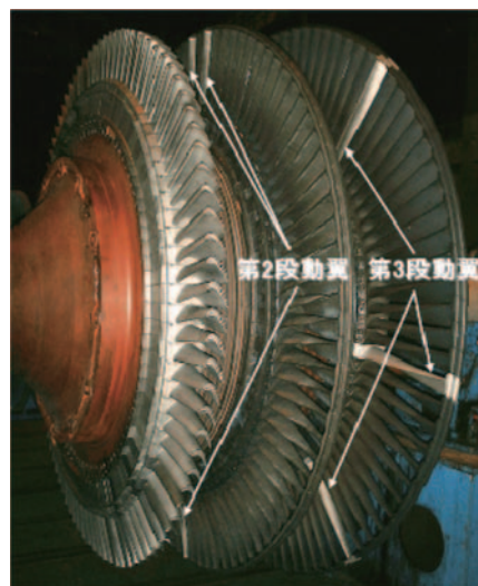
Fig. 1 Appearance of the treated blades installed in the turbine rotor before trial operation (1) .
