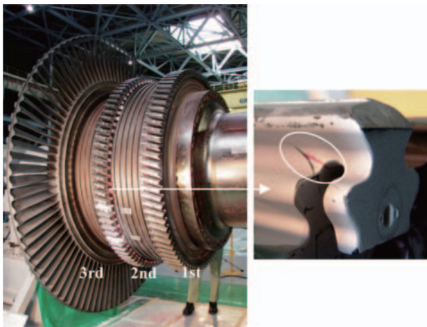
Fig. 2 Appearance of the gas turbine rotor and the part of the "lock wire tub" (9) .
