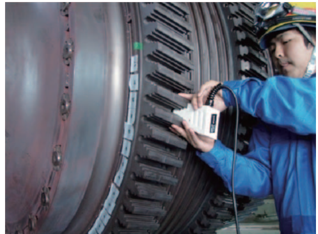
Fig. 3 Eddy Current Inspection of a gas turbine rotor.
