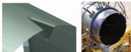
Fig.1 Concept of notch (left) and the 6-notched nozzle (right).
